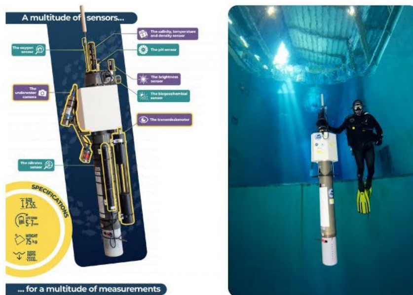
Figure 3: A biogeochemical float with its 6 additional sensors (left). Argo biogeochemical float at the Ifremer facility (right). Source: Euro-Argo. Graphic credit: ERC REFINE. Photo credit: Olivier Dugornay.
